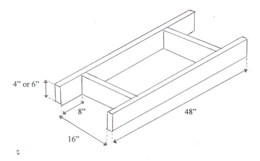
This is a very simple hive stand that will hold one or two hives. It should not be placed directly on the ground, but rather should be placed on top of bricks, concrete, or construction blocks.
